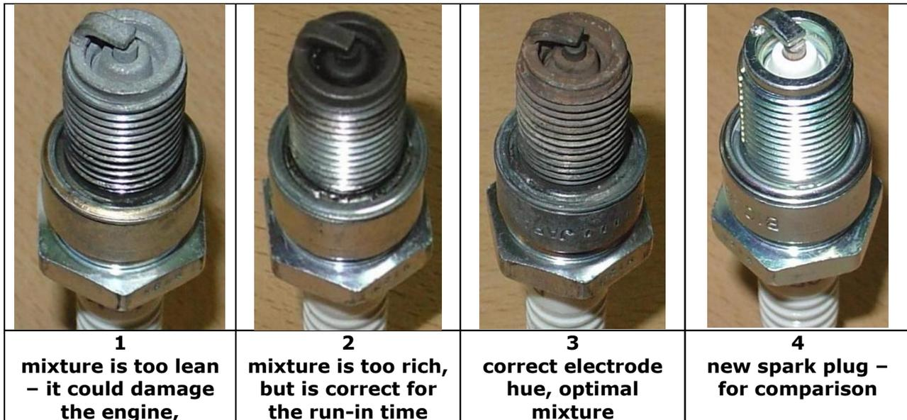
☞ During the run-in time a wet and tarry spark plug is a good sign because it means that the mixture is rich. Petrol in a two-stroke engine is not only a fuel but also a warmth conductor, which is emitted excessively during the run-in. During the run-in time, we even advise you to use a too rich mixture at the expense of slightly weaker engine performance.
