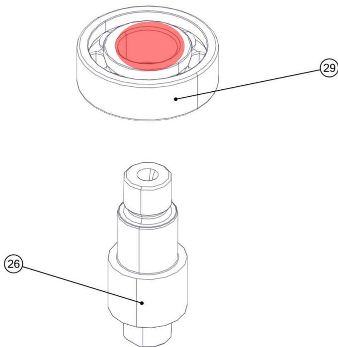
Fit the O-ring (28) on the pinion (26).
