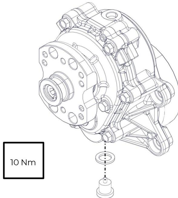
Remove the front screw with the copper seal.
