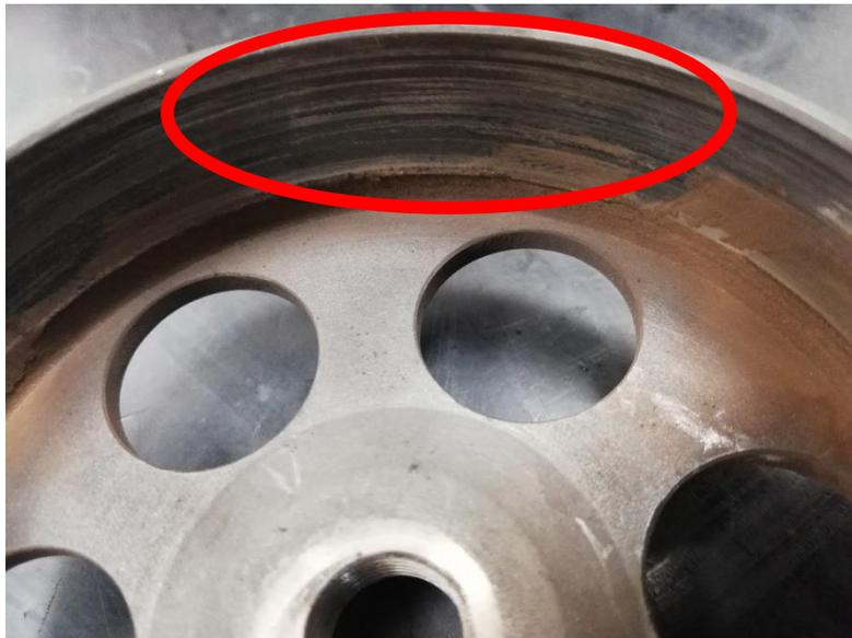
Measure the internal diameter of the clutch bell, the table shows the factory settings.
