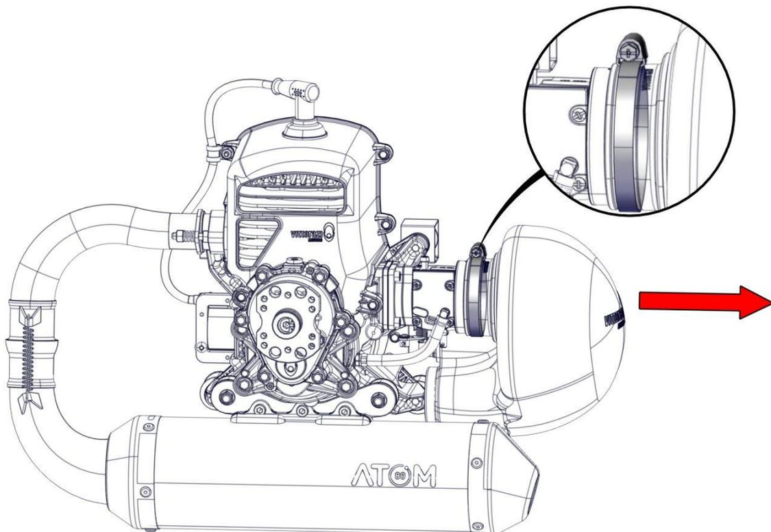
Fold the sleeve inwards and remove it from the airbox.
