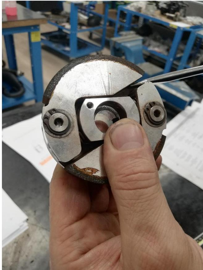
Check the bushing of the transmission cover: the side surface must be smooth and free of signs of wear, otherwise (as in photo) it must be replaced.
