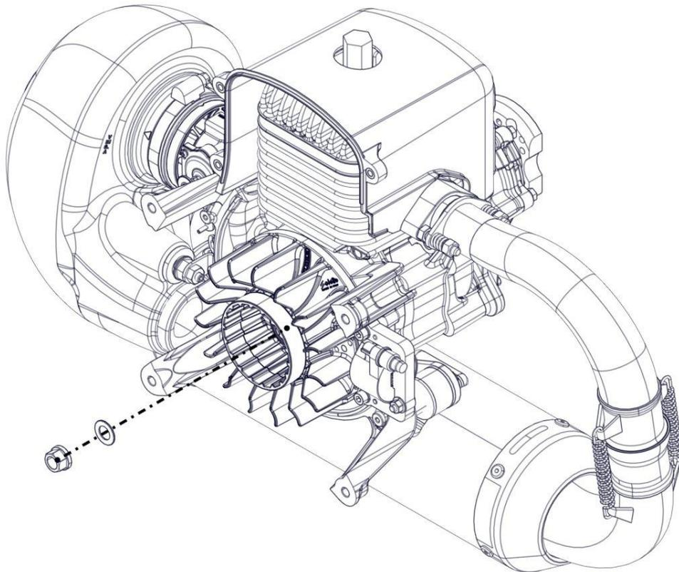
Screw the flywheel extractor into the starter cup.
