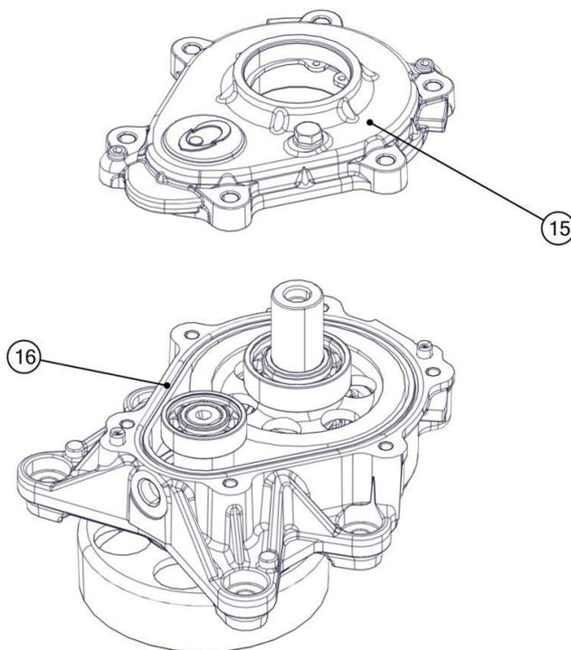
Insert and pre-tighten alternately the 2 highlighted flanged head screws M5x20.
