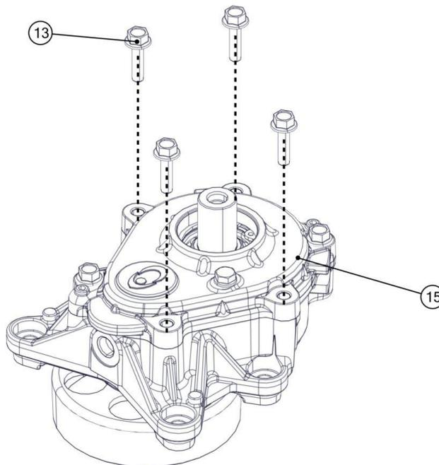
Pre-tighten progressively, then tighten in crosswise order to 6,5 Nm.
