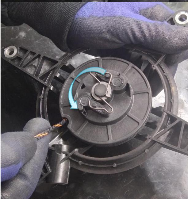
Hold the pulley and wind 4 turns of rope counterclockwise.
