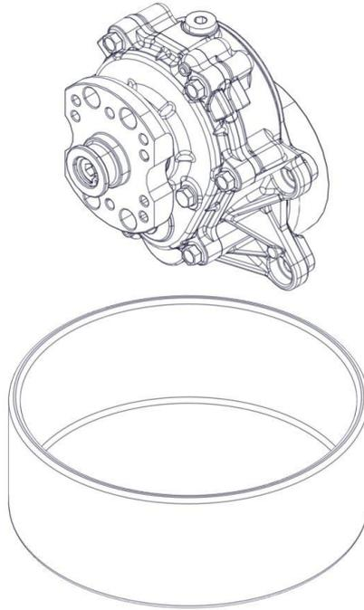
Hold the engine upright and remove the lower cap with the copper seal.
