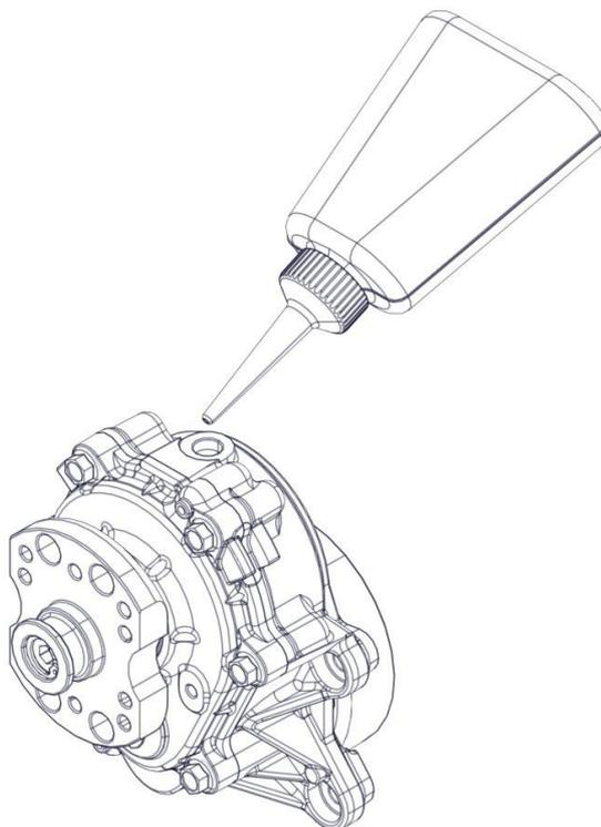
Fill the oil until is leaking from the front hole.
