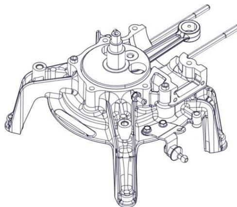
Heat the transmission side crankcase to 120 °C.
