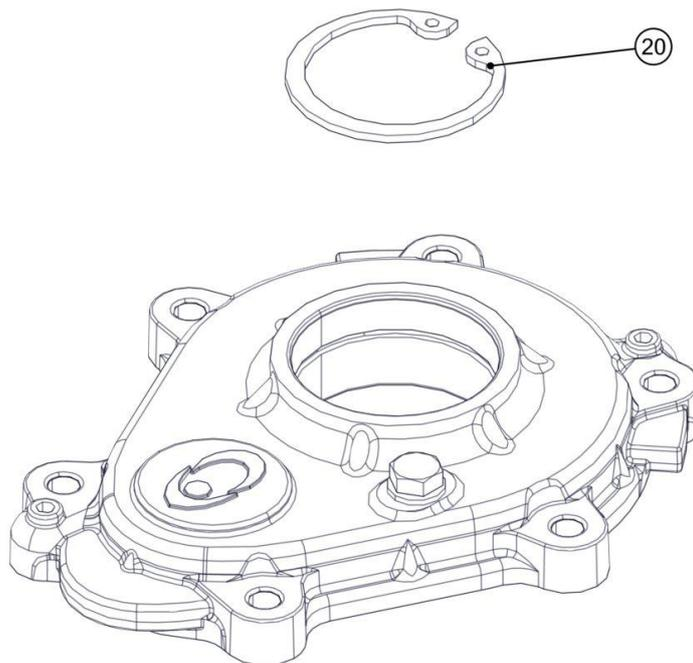
Heat the cover at the bearing seats at 120 °C.
