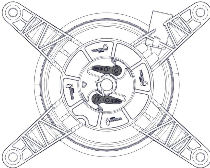
Insert the 4 rubber mountings into the manual starter bracket (2).
