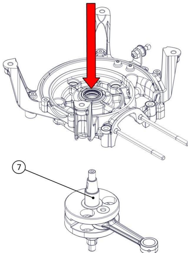
Heat the manual starter side crankcase to 120 °C.
