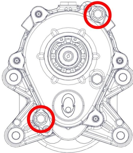
Insert the remaining 4 flanged head screws M5x20 (13) into the cover (15).
