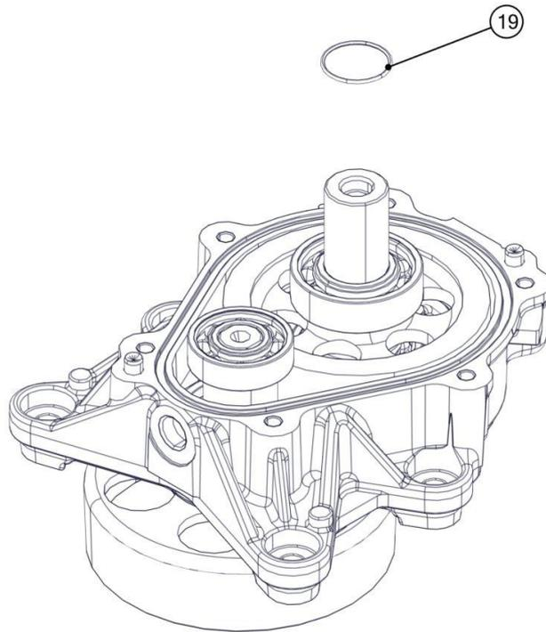
Insert the O-ring (16) between on the gearbox.
