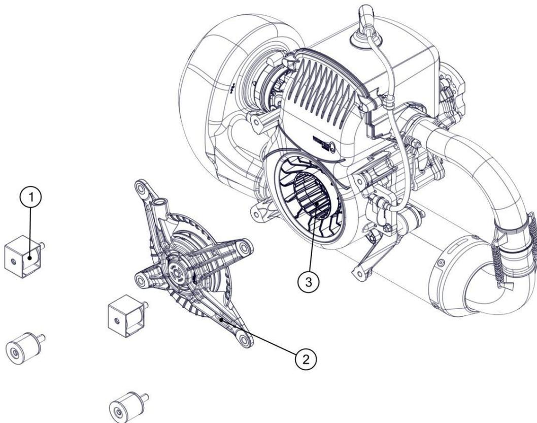
Insert the rope into the guide eyelet of the handle and tie a knot to prevent it from slipping out. Pull the handle and check that the pulley rotates smoothly without blocking.
