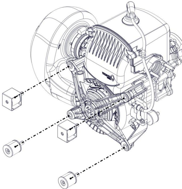
Remove the 2 rubber mountings of the exhaust system.
