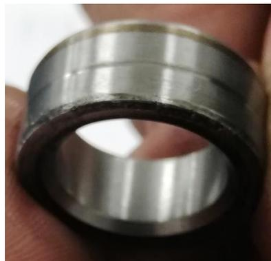
Check the 4 bearing seats: there must be no polished areas. Also measure the diameter of the 4 seats, the table shows the factory settings.
