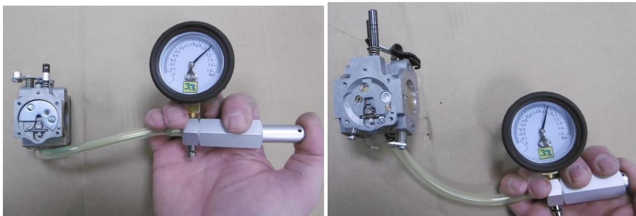
In the event of a fault, measure the height of the metering lever again and replace the spring (17) if necessary.
