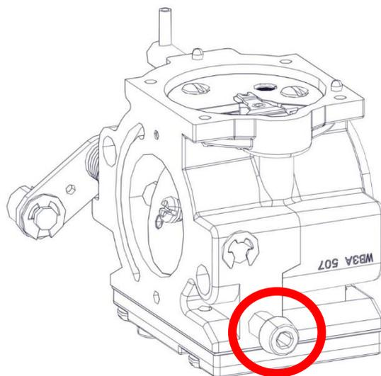
Set a pressure value lower than the values in the table and check that the needle of the metering lever does not allow air to escape. Carry out further tests by gradually increasing the pressure.
