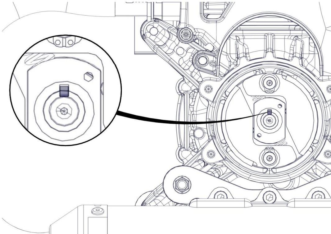
Insert the nut M10x1,25 (34) with the washer (35) and tighten to 52 Nm.
