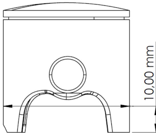
Measure the diameter of the cylinder at 10 mm from the top.
