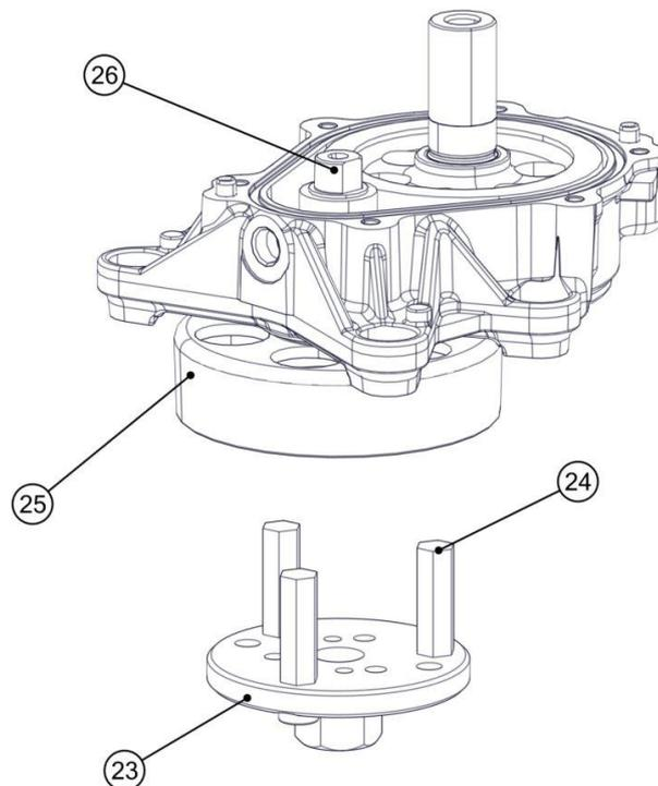
Remove the pinion (26) using an awl (27).
