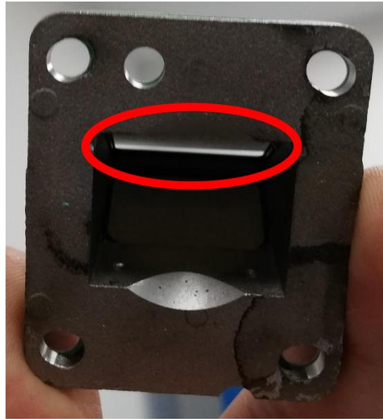
If the previous checks are not passed or if routine maintenance is required, replace the petals.
