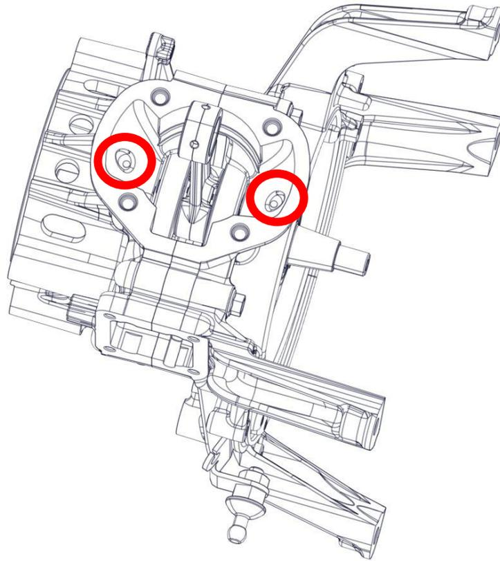
Check the sliding of crankshaft on the bearings.
