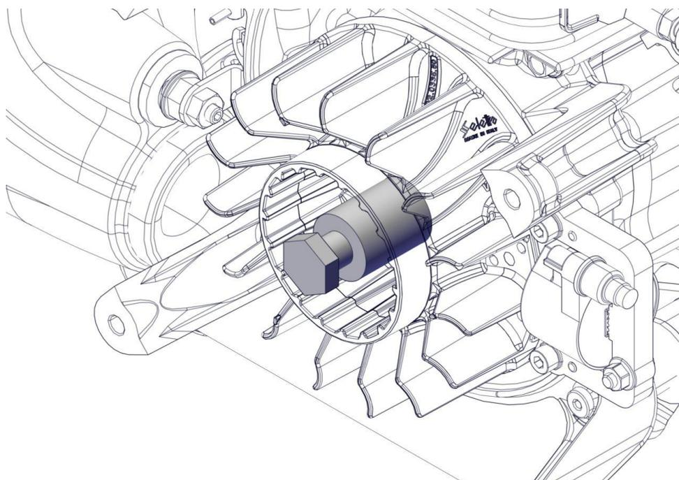
Turn the central pin of the extractor until the flywheel is removed from the crankshaft.
