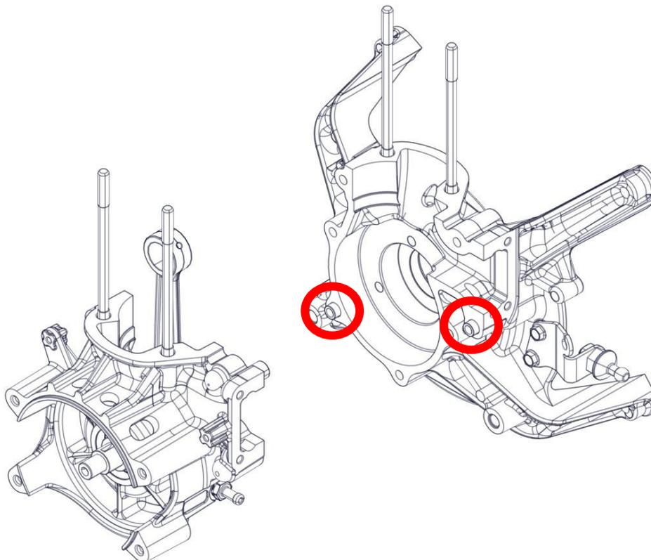
Insert the 7 flange-head screws M5x40 (1) and tighten with the torque shown in the figure.
