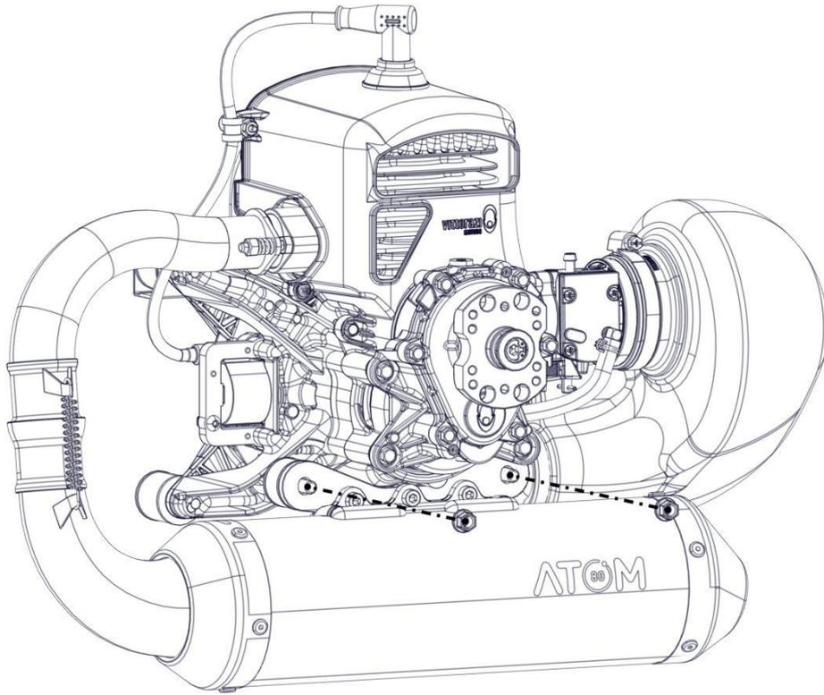
Remove the 2 self-locking nuts M6 and 2 springs from the exhaust studs.
