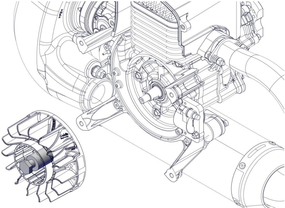
Remove the 2 Allen screws M5x20 (7) with washers (8) and the coil (9).
