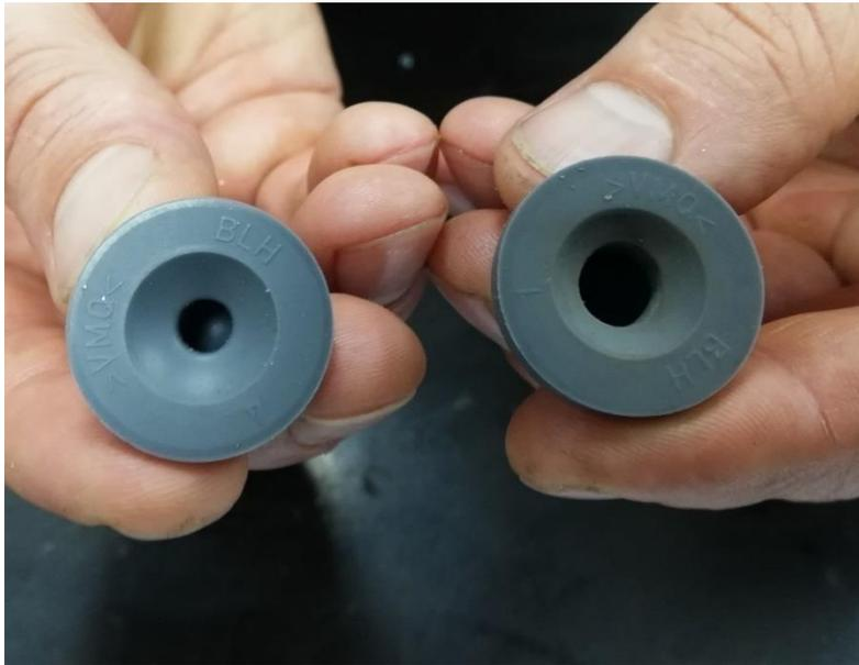
Check the Venturi: it must be firmly attached to the airbox and have no play in the seat.
