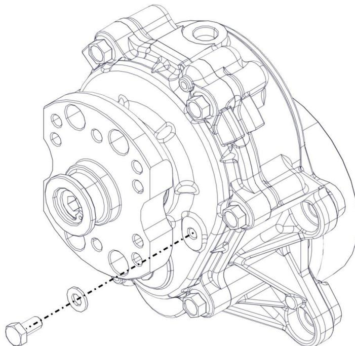
Fill the transmission with the specific oil (Maconoil Supermoly 220 with 3,5 % Mos2). Vittorazi supplies 30 ml bottle (AT160) that is required to fill completely the transmission box.
