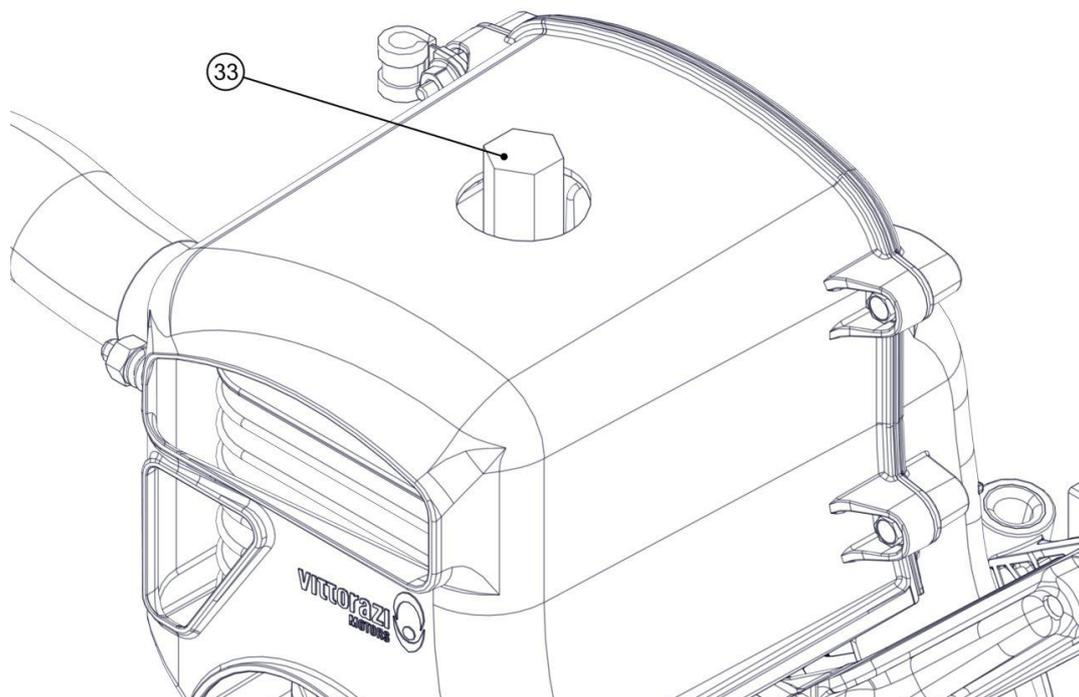
Turn the clutch until the piston is in contact with the piston lock.
