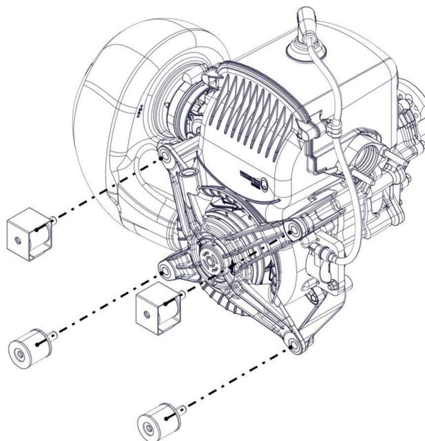
Insert the 2 rubber mountings of the exhaust system.
