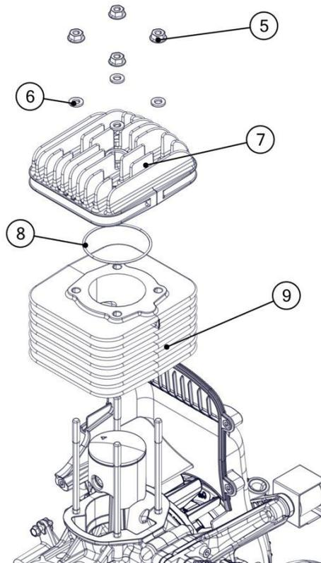
Tighten the nuts progressively, then cross-tighten to 10 Nm.
