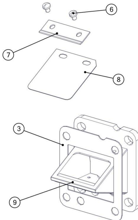
Place the reed valve (4) with the gaskets (3) on the crankcase (5).
