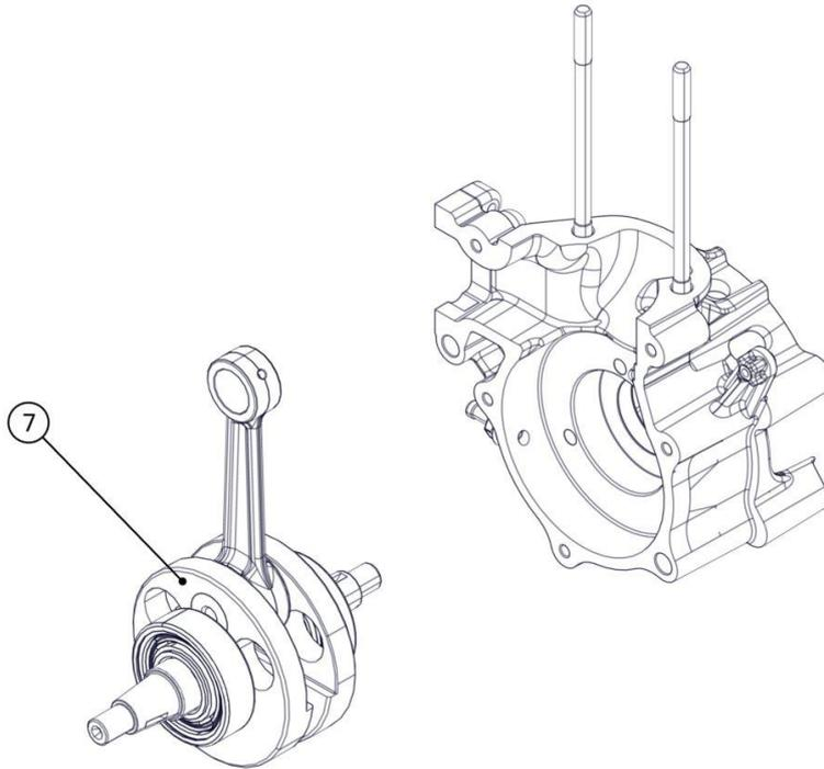
Heat the manual starter side crankcase to 120 °C.
