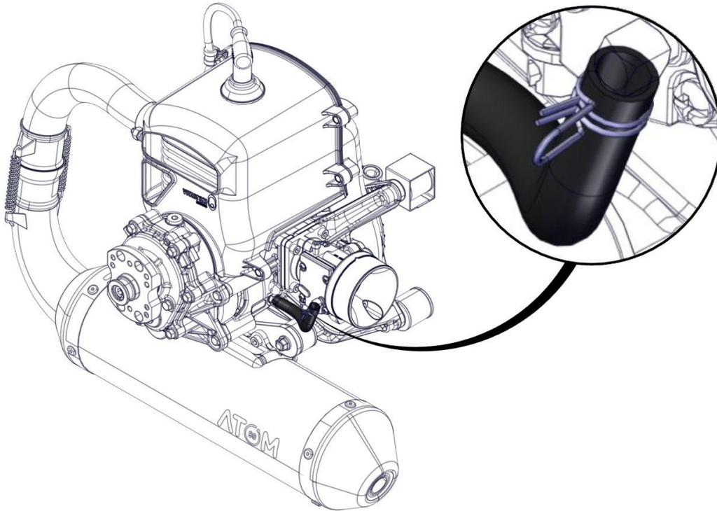
Remove the 2 Allen screws M6x60 (1) (M5x70 with washers for WG8) from the airbox connector (2).
