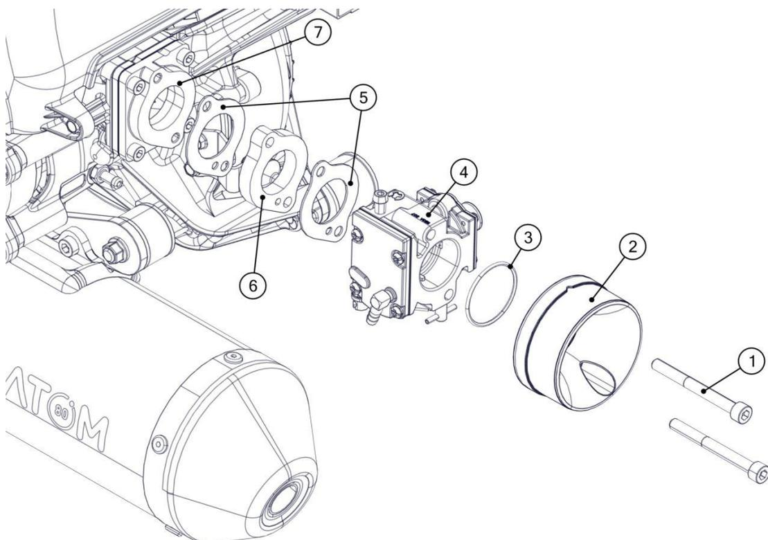
Disassemble the carburettor by removing the components shown in the figure.
