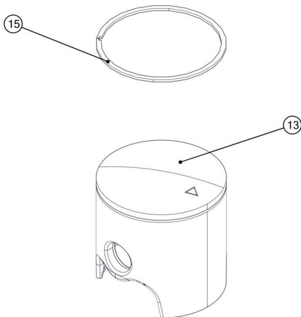
Insert the circle clip (16) on the piston (13) on the manual starter side respecting the position shown in the photo.
