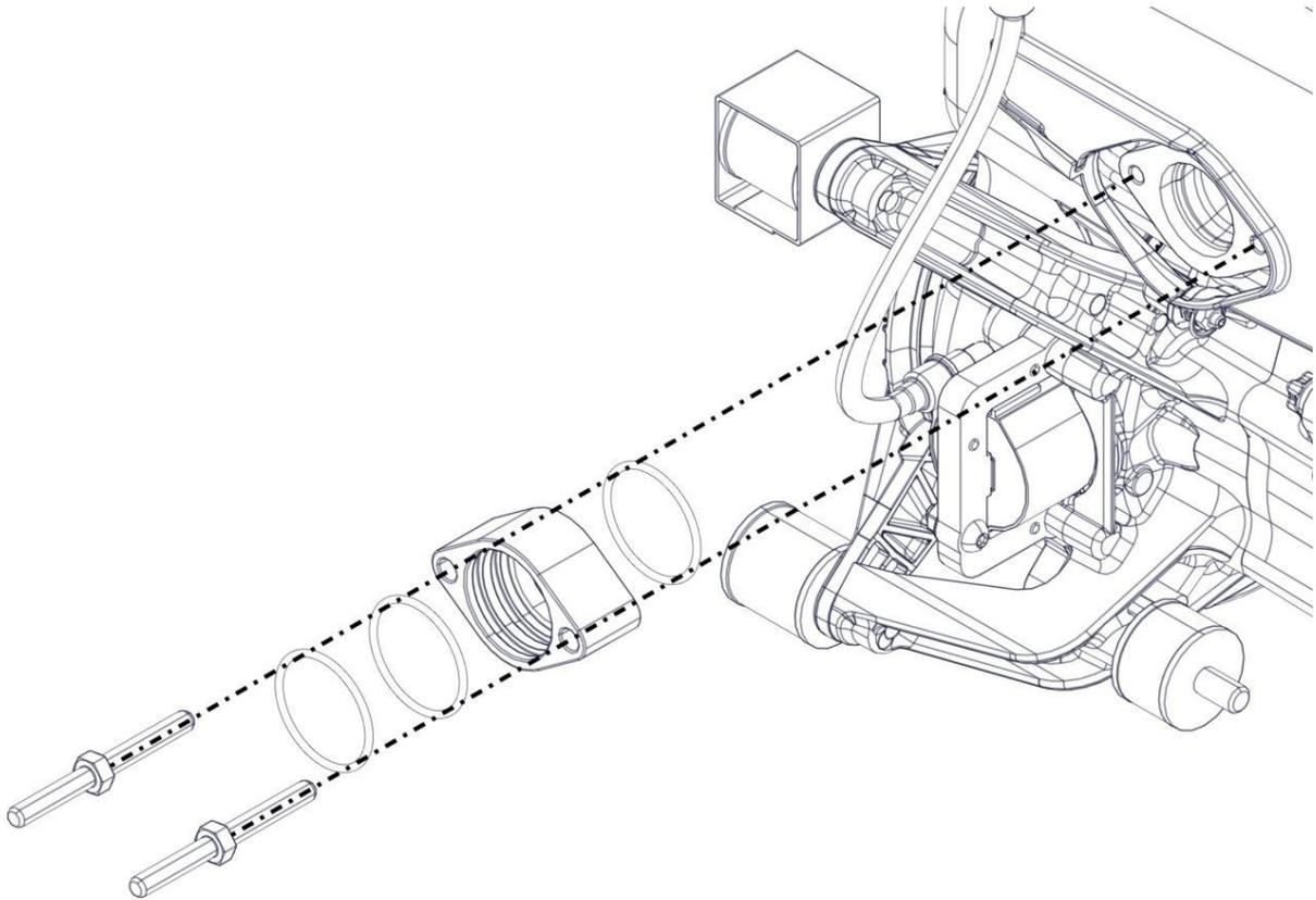
Remove the 2 safety cables around the springs of the coupling.
