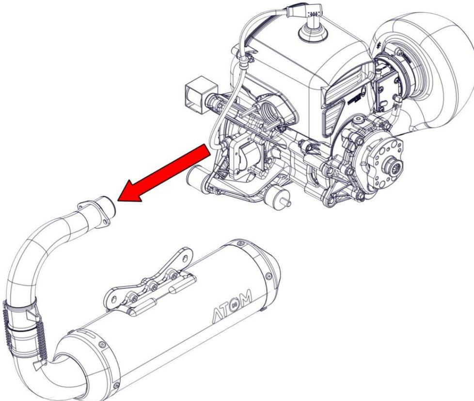
Remove the 2 studs M6 and the bushing.
